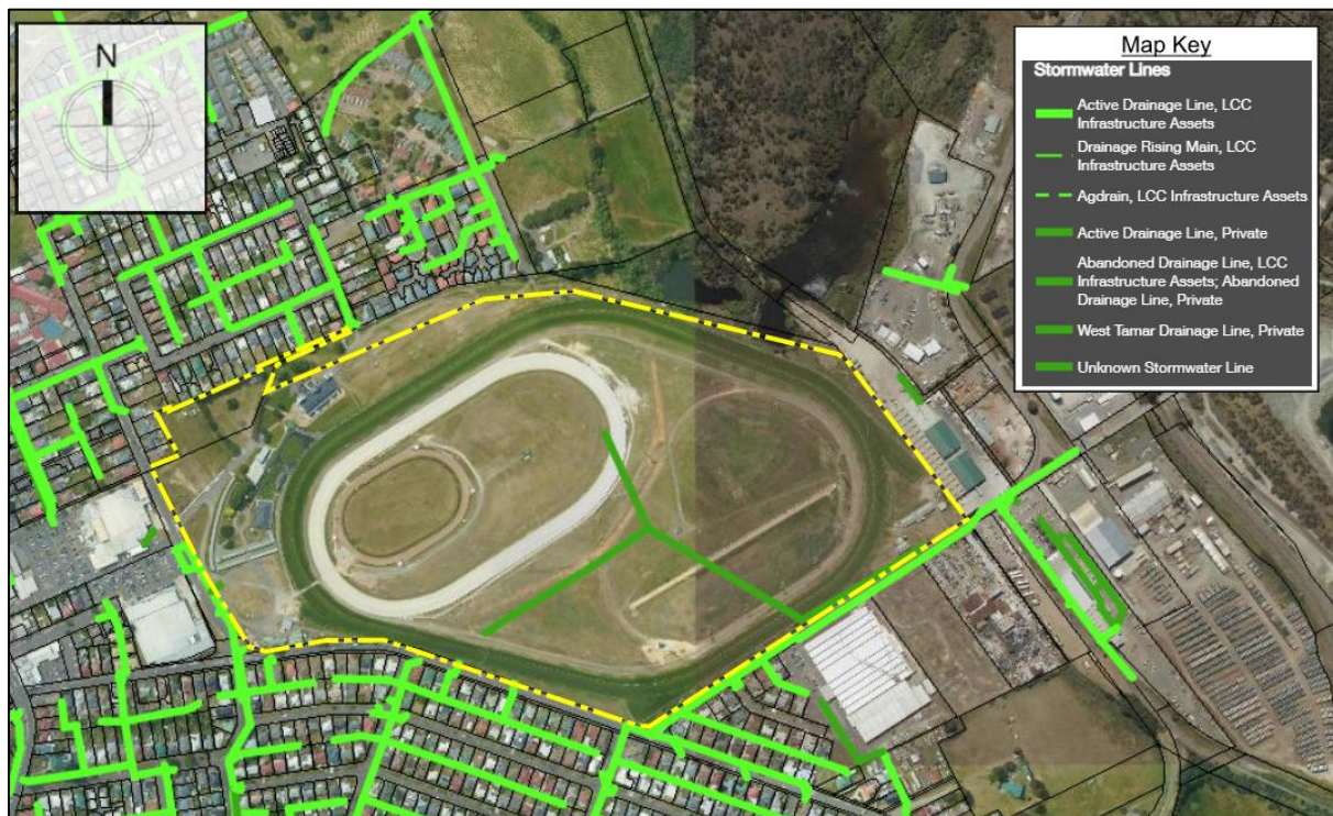
Figure 11 - extent of public stormwater system.
