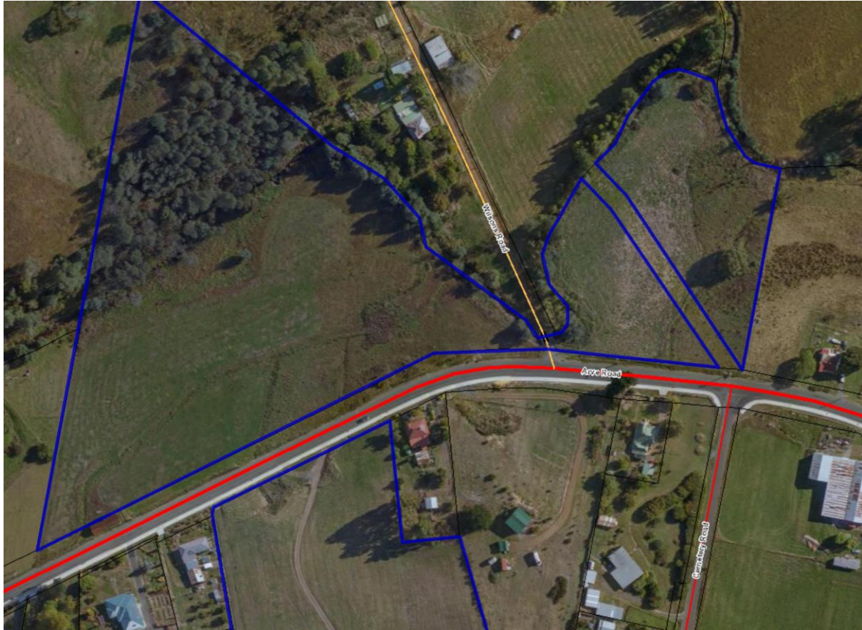
Figure 1.1b – the lot boundaries are shown in blue, with Wilsons Road (yellow) crossing through the title of the lot whilst the road reserve is through the center of the adjoining paddock. (Source LIST Map)
