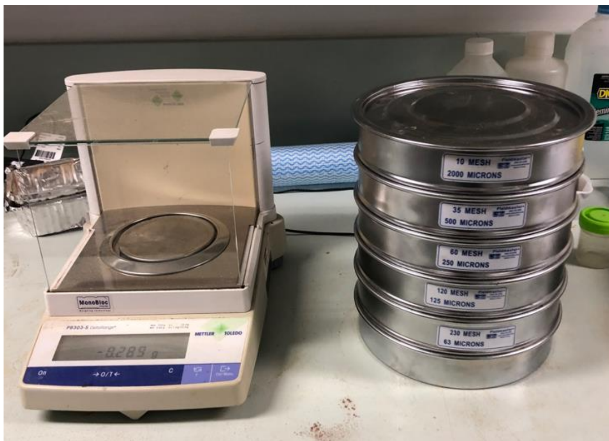
Standard set of sieves using -1 \phi (gravel) and 1 \phi to 4 \phi (coarse sand to silt) and sediment retained was weighed.
