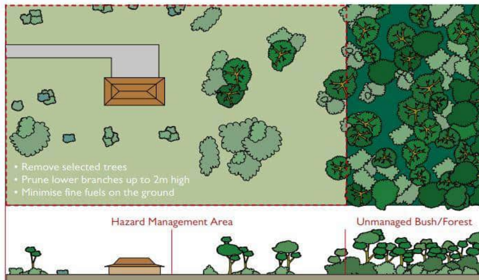
Figure 4 - Example Hazard Management Area
