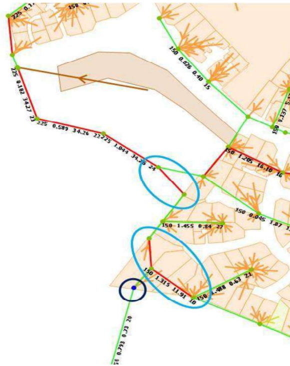
Figure 1: Pipes exceeding capacity after the introduction of the proposed development, are circled in BLUE. Overflowing MH after the introduction of the proposed development, is circled in DARK BLUE.
