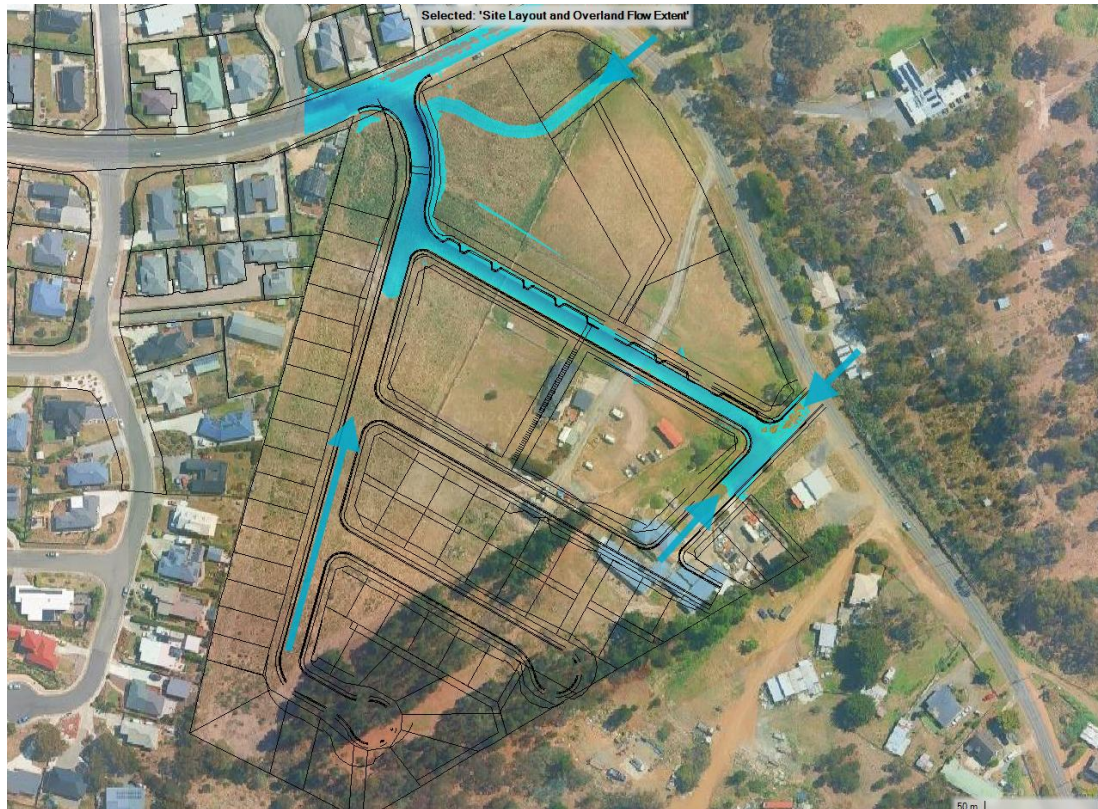
Figure 22 - HEC-RAS - Site Layout and Overland Flow Extent
