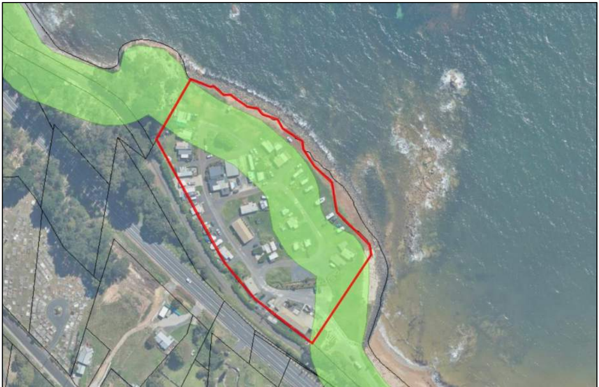
Figure 43: Extent of the waterway and coastal protection area guidance map, indicating a 40m buffer from the high-water mark (source: www.thelist.tas.gov.au © State of Tasmania).
