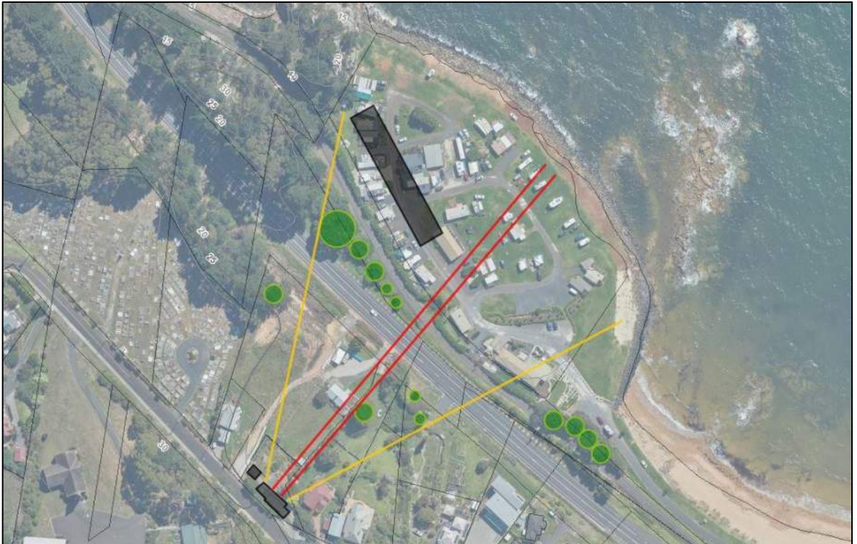
Figure 36: Approximate view lines/view-field from 1B Main Road. Red line indicates primary view orientation. Orange lines indicate an approximate field of view. Green circles indicate existing vegetation. Black area indicates approximate 4-storey building location (source: www.thelist.tas.gov.au © State of Tasmania)
