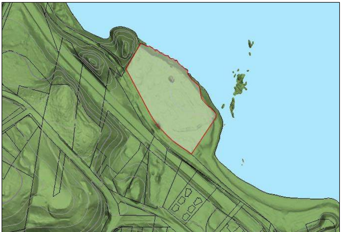
Figure 4: Hill shade map with cadastre and 5m contours (Source: www.theLIST.tas.com.au © State of Tasmania)
