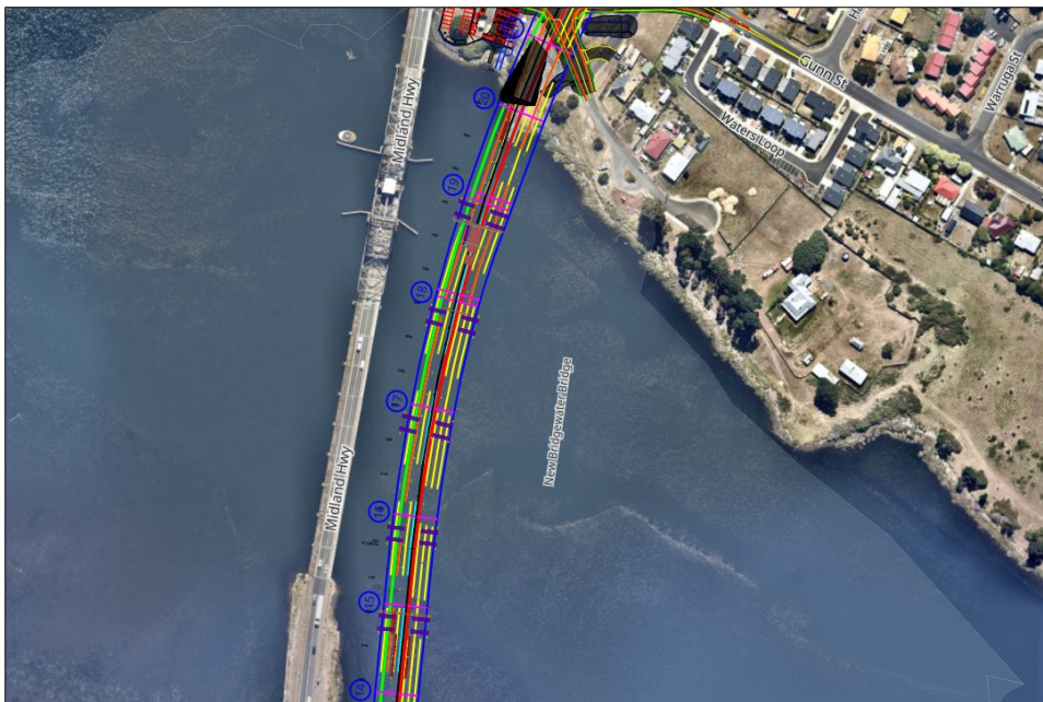
Figure 16 - Extent of Temporary Bridge
