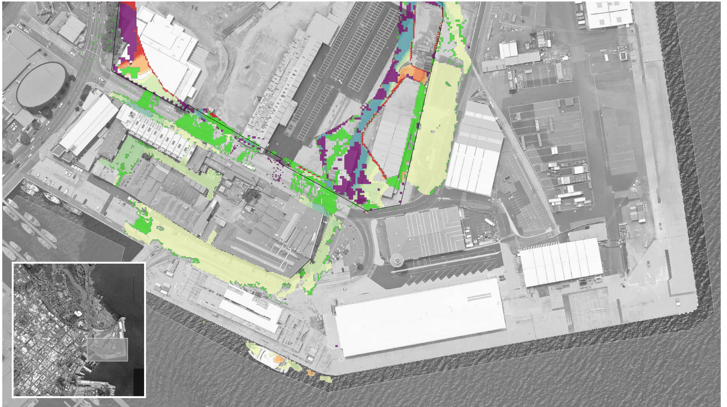
Figure 10.2: Water Level Afflux - 10% AEP 2100 Existing Condition 2 and Option 3
