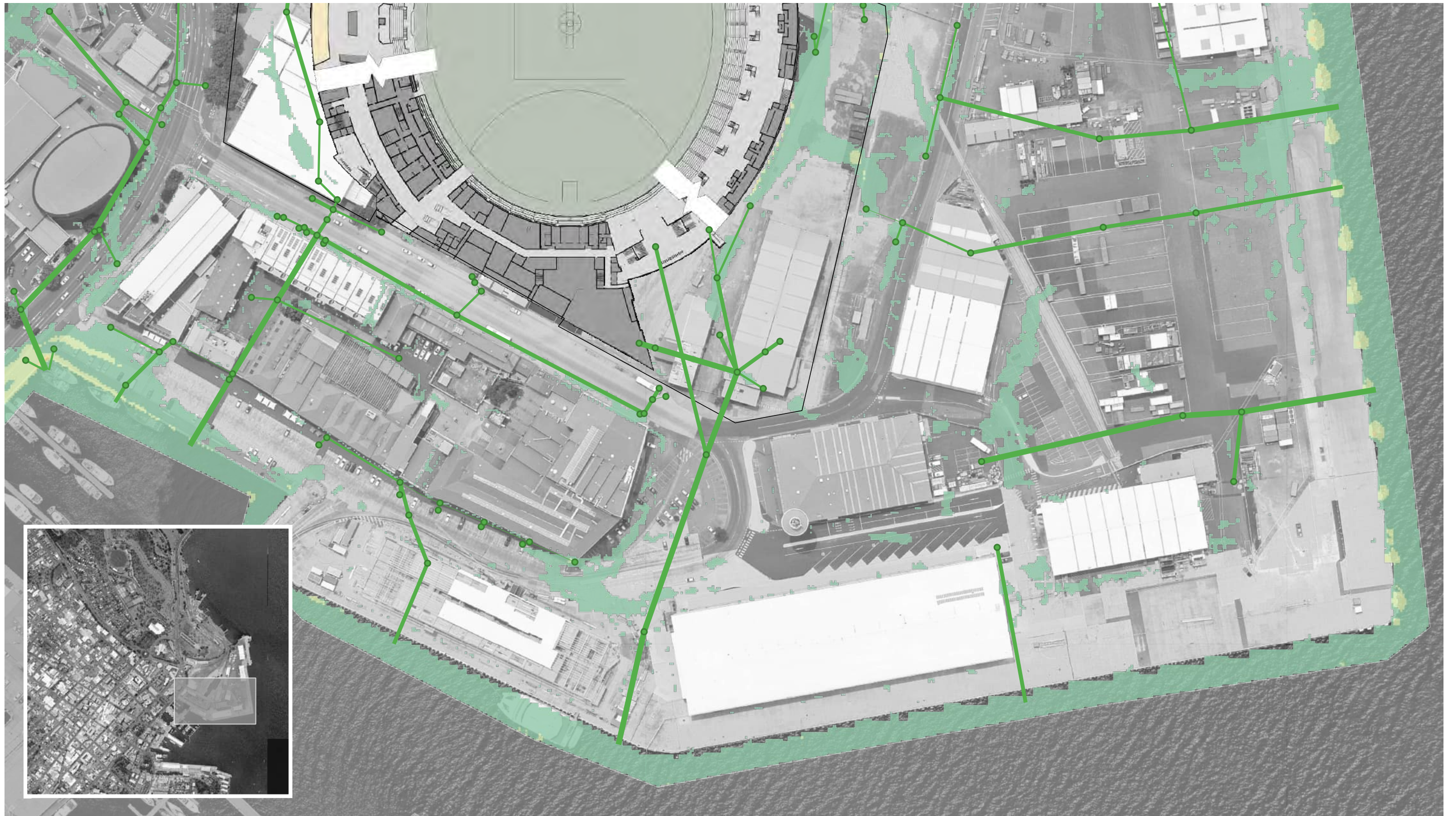
Figure 71.2: Peak Velocity - 1% AEP 2100 Option 3: Stadium roof drainage connection to the East and South.
