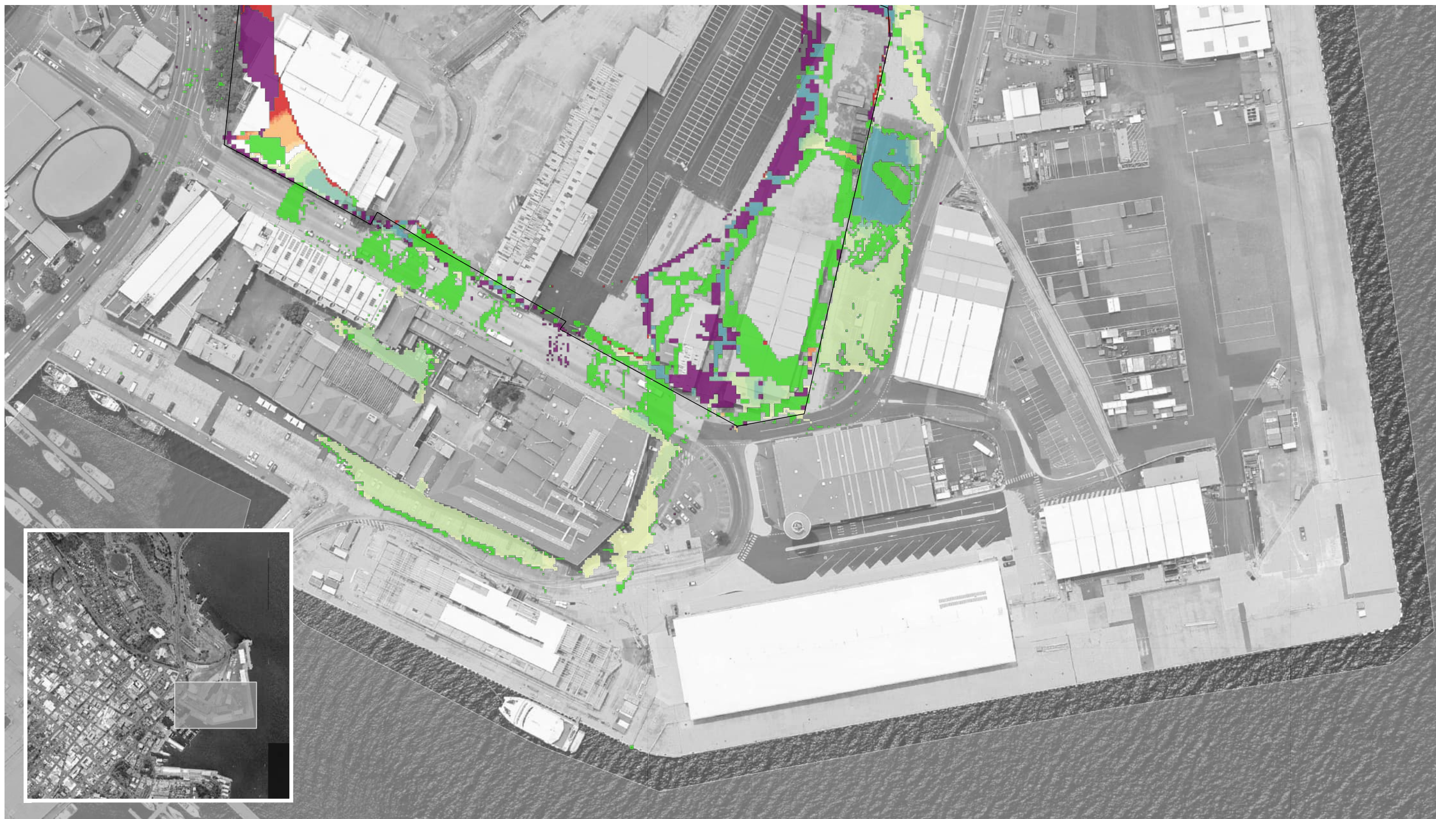
Figure 24.2: Water Level Afflux - 1% AEP 2030 Existing Condition 2 and Option 2
