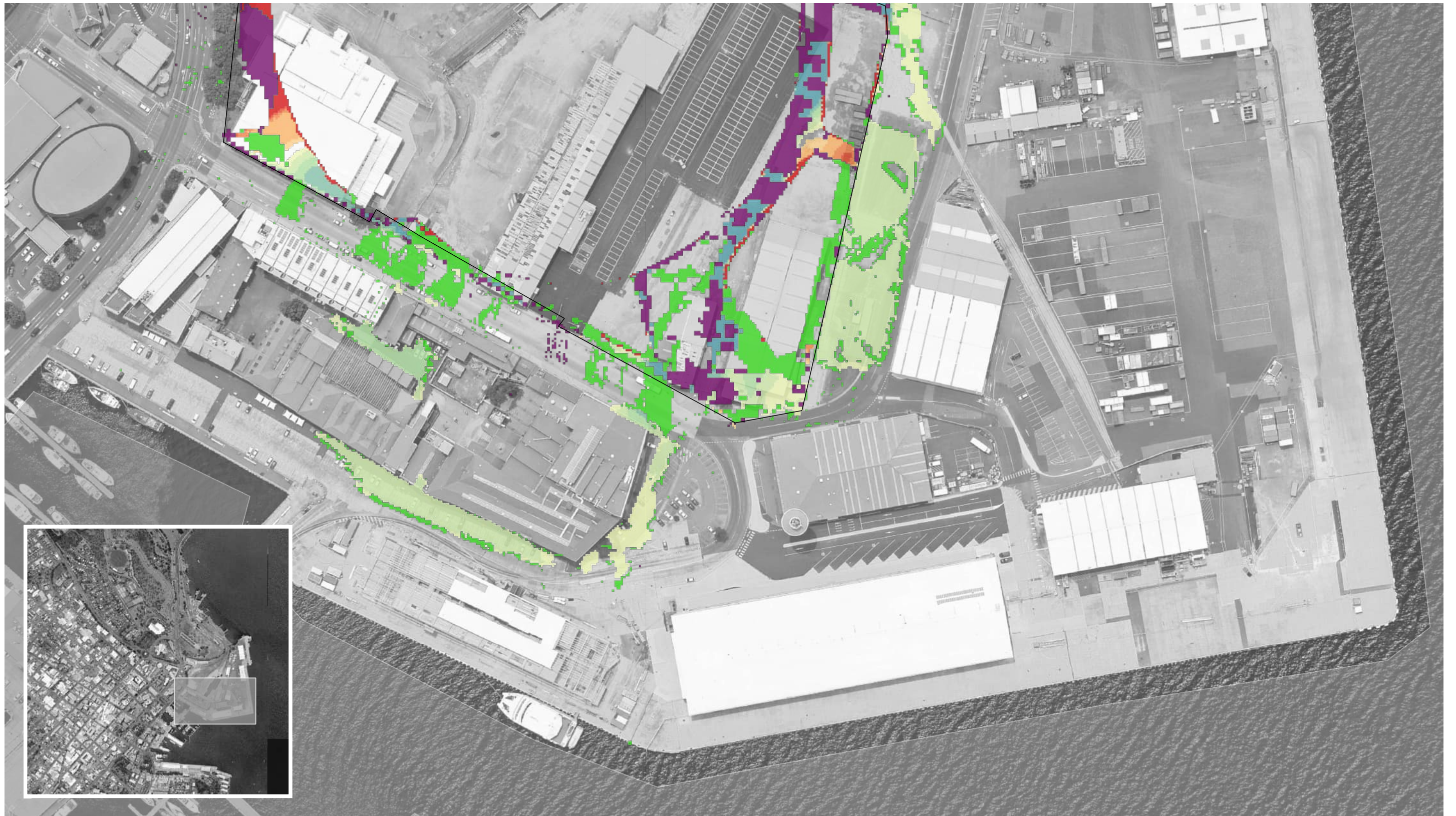
Figure 52.2: Water Level Afflux - 10% AEP 2030 Existing Condition 2 and Option 3
