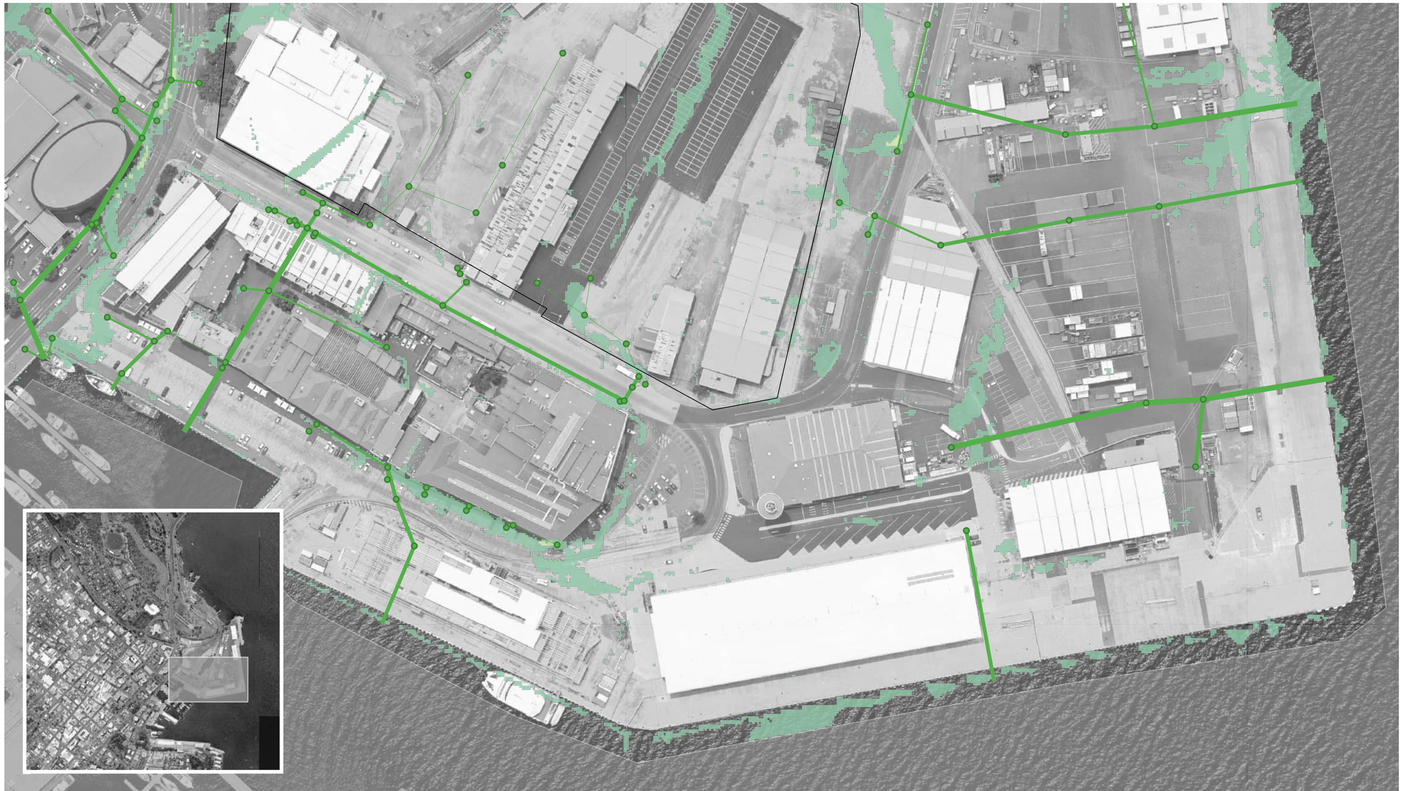
Figure 29.2: Peak Velocity - 10% AEP 2030 Existing Condition 1: Pre-2020 access road construction.
