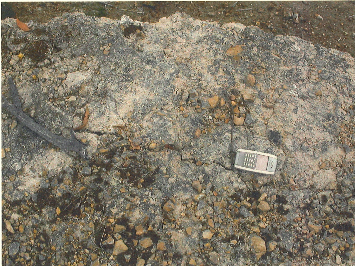
Plate 13 Tension crack in an overhanging area near the edge of the upper bench of the quarry
