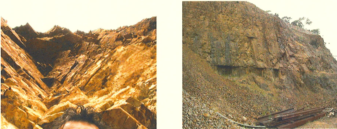
Plate 10 Sections of quarry face with overhangs of rock.
