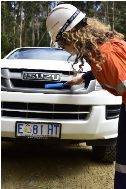
Cleaning the radiator grill with dry brush
