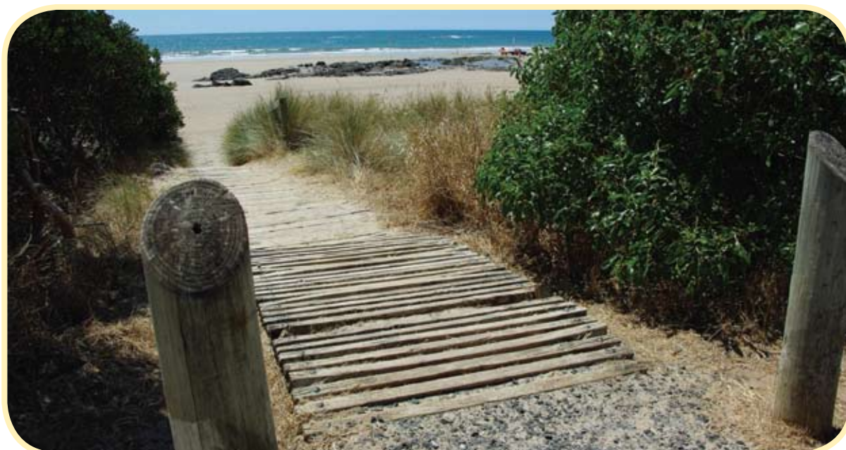
Figure 13.13 Pedestrian sand ladder minimises erosion of the dune. © Leah Page
