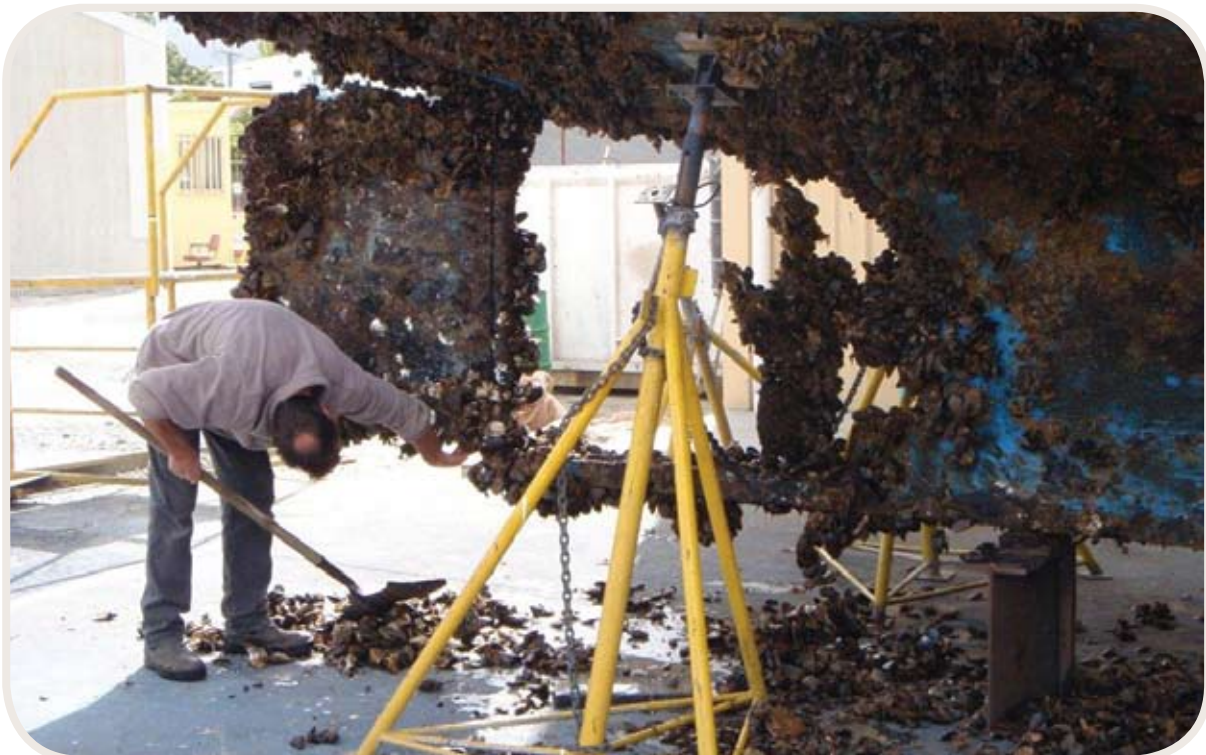
Figure 10.14 Boat hull cleaning removes marine pests but the wash water needs to be contained and treated at the boat facility, such as here at the Clean Lift facility at Prince of Wales Bay. © Ruth Eriksen
