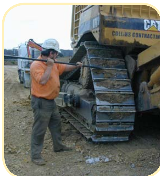
Figure 13.2 Cleaning soil and plant material off vehicles before entering and leaving sites will minimise spread of weeds and diseases. © Forestry Tasmania
