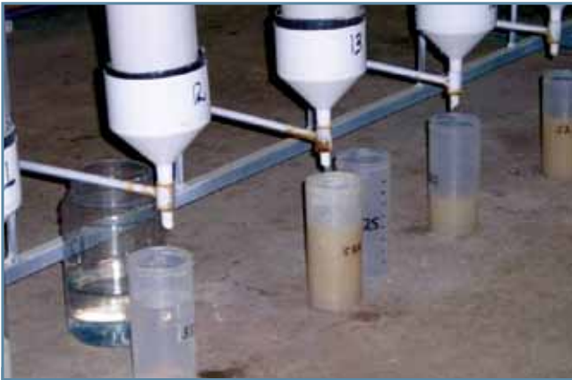
Figure 39. Pinhole test for compacted soils & fill. (Photo, Raine & Loch 2003).
