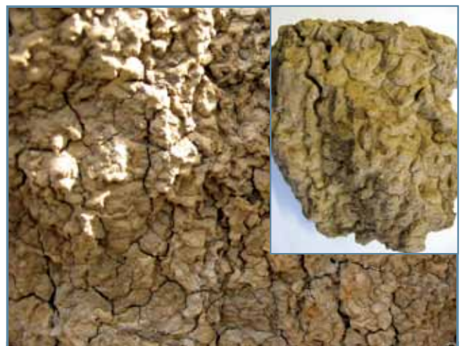
Figure 9. (a) Example of dribble pattern on an exposed subsoil, the photograph was taken from within an actively eroding tunnel system. (b) Dribble patterns on sodic soil ped.
