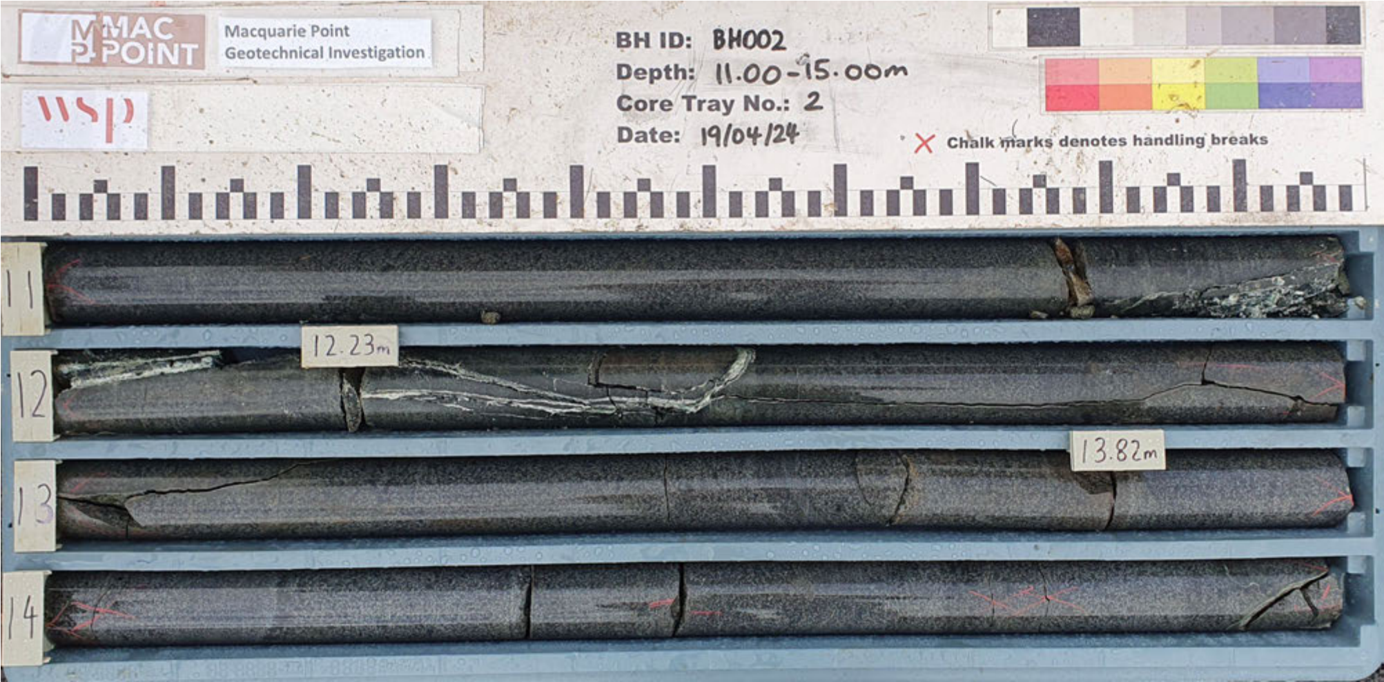
PointID : BH-002 Depth Range: 11.00 - 15.00 m
