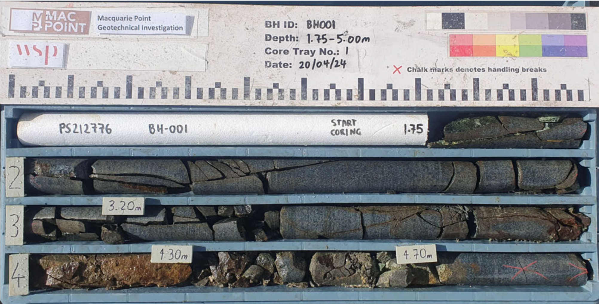
PointID : BH-001 Depth Range: 1.75 - 5.00 m
