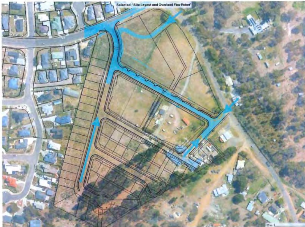
Figure 22 - HEC-RAS - Site Layout and Overland Flow Extent
