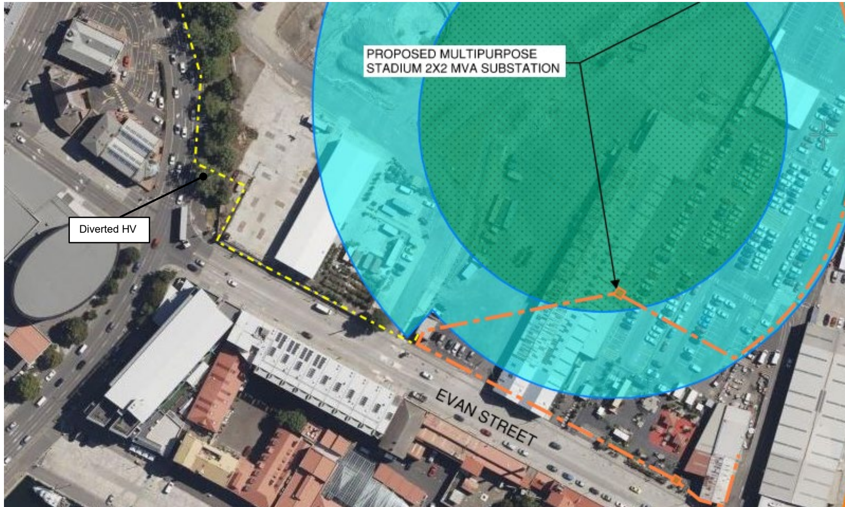
Figure 12 -Substation Upgrade (Subject to Survey & Locating)
