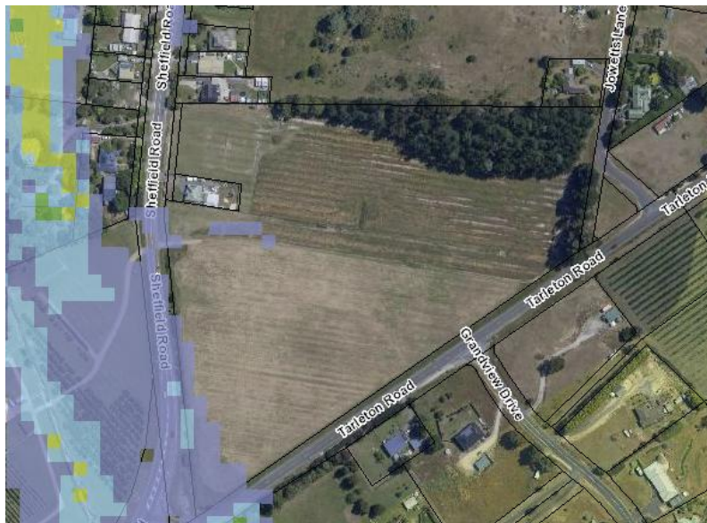
Figure 16 1.0% AEP Hazard Overland Flood Mapping (Climate Change).
