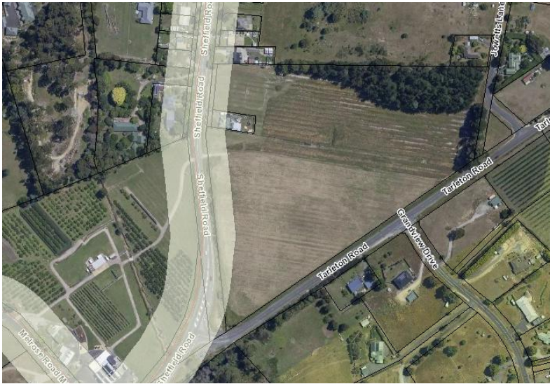
Figure 21 TasGas pipeline (red) and buffer area (beige)
