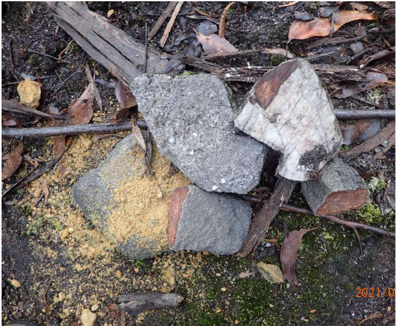
Plate 19. Example of different rock types from a small area (ca. 2 m radius) in the northeast corner of the title, showing pebble-rich sandstone, a finer-grained mudstone, lump of pure quartzite and highly weathered sandstone that crumbles to coarse sand
