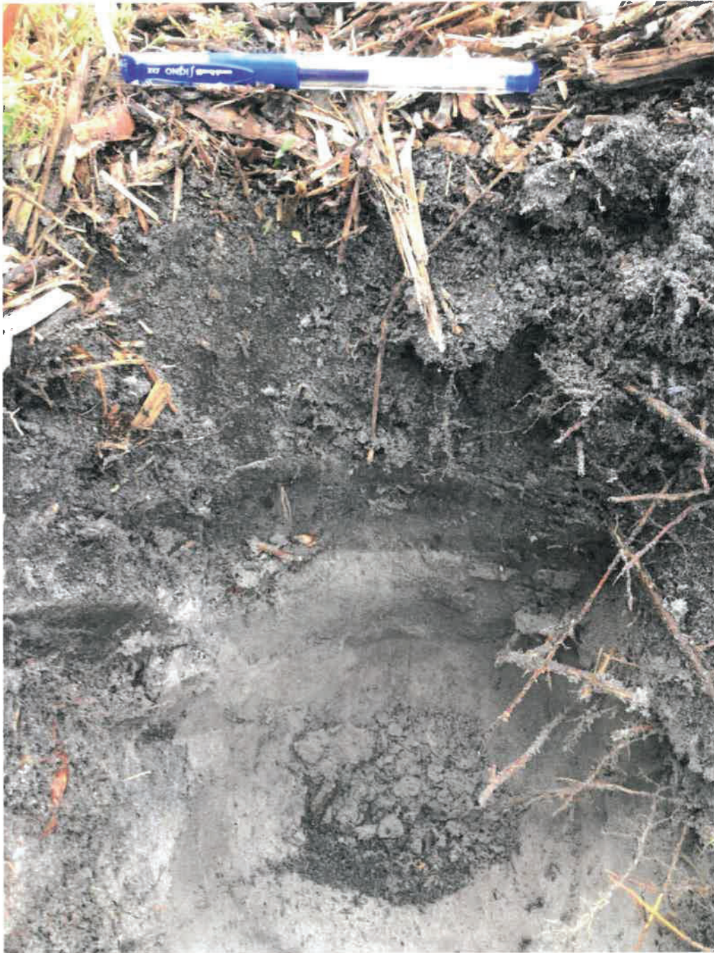
Figure 6 Grey podosol soil profile present throughout much of the property (taken on the site assessment 1/3/2022)
