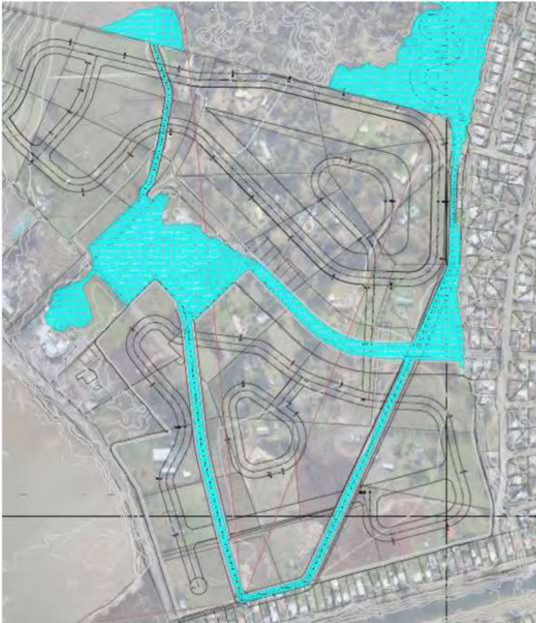
Figure 3-9 - Inundation extent for a 1 in 100 year ARI rainfall event with year 2100 rainfall intensities and Mean High High Water (MHHW) sea levels (1.1m AHD). Note that the only residential area effected is Roches Beach Living.
