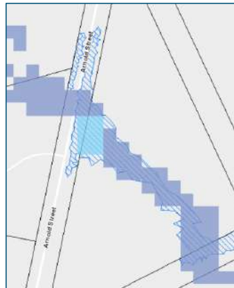
Figure 31 Showing hazard area of H2 (light blue) and H1 (remaining darker blue)(Land Tasmania 2021)
