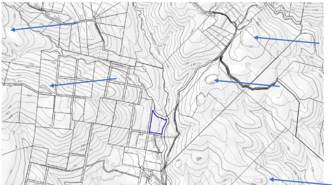
Figure.7. Topographical mapping from theList with each line representing a 10m contour. Peaks to the west and east are indicated with blue arrows. The subject site is outlined. The subject site is located closely to Browns River which runs through the valley. Source: TPC, sourced 4 November 2024, no nominated scale.
