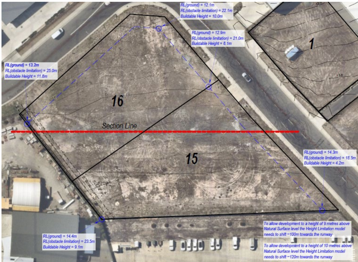
Plan 2 – Revised OLS mapping 7 & 9 Cherokee Drive (Source: Rogerson & Birch Surveyors)
