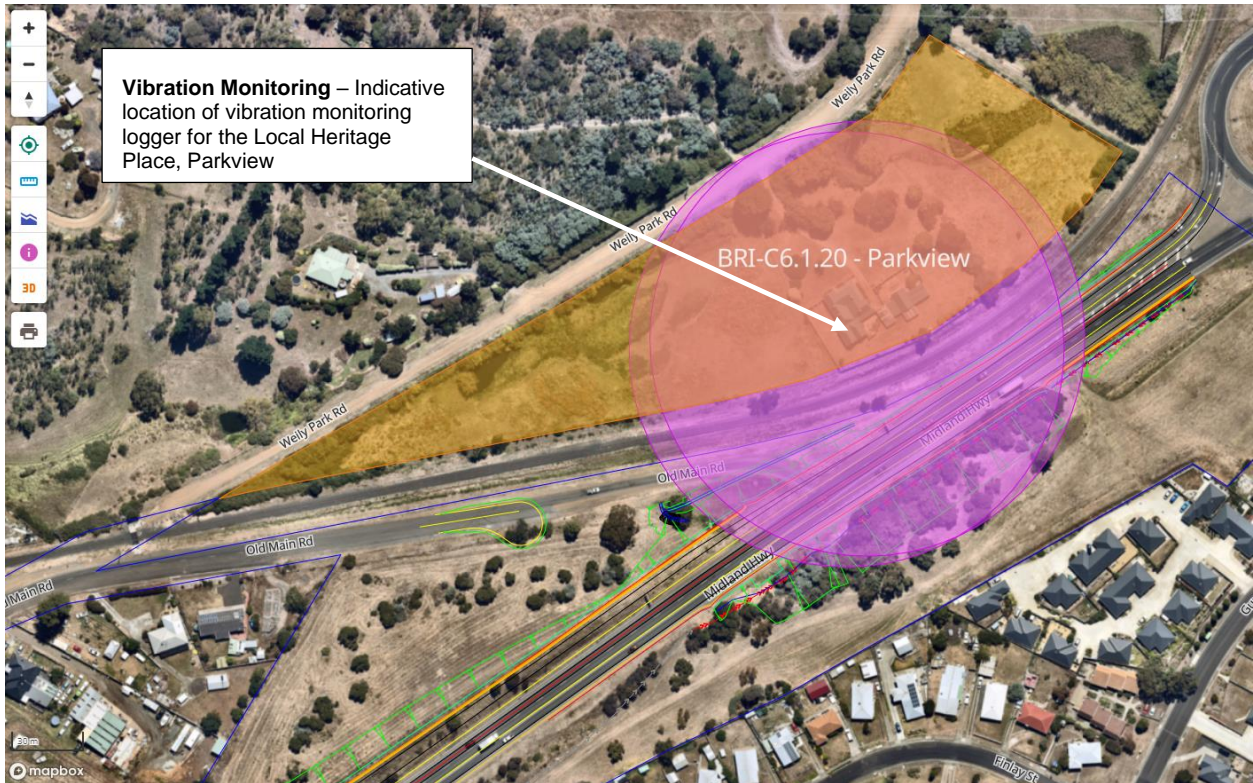
Figure 9: Indicative 90m Vibration Management Zone (purple circles) for 20t vibratory rollers working in the vicinity of Parkview. Where works are required within these distances, the mitigation measures listed in Section 8 of the CNVMP will be applied where reasonable and feasible, including installation of a continuous vibration monitoring logger. Source: Map from Civillo 02-Nov-2022.
