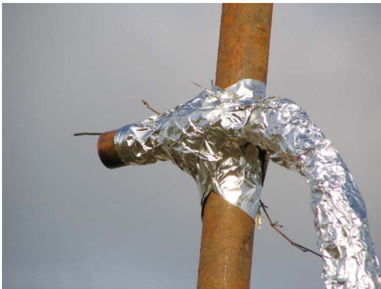
Figure 10 Typical radiometer and thermocouple mounting on poles
