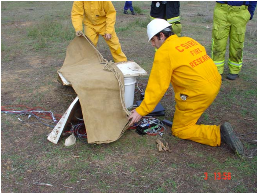
Figure B1. Crude but effective protection of data logging equipment
