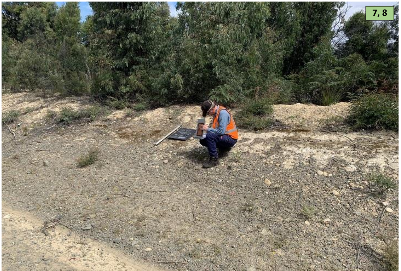
Site D36 (above). Permian-age feldspathic sandstone weathered to a light brown silty clay. Sand 10%, silt 20%, clay 70%. Tested sample: Emerson Class No. 7 or 8 (no dispersion).
