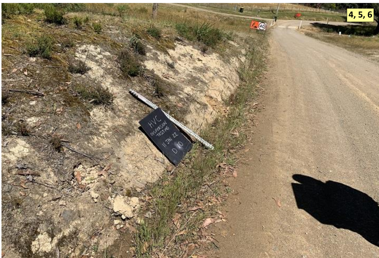
Site D10 (below). Yellow-white coloured Permian-age siltstone weathered to a clayey silt. Clay 30%, silt 70%. Tested sample: Emerson Class No. 4, 5 or 6 (slight to no dispersion).
