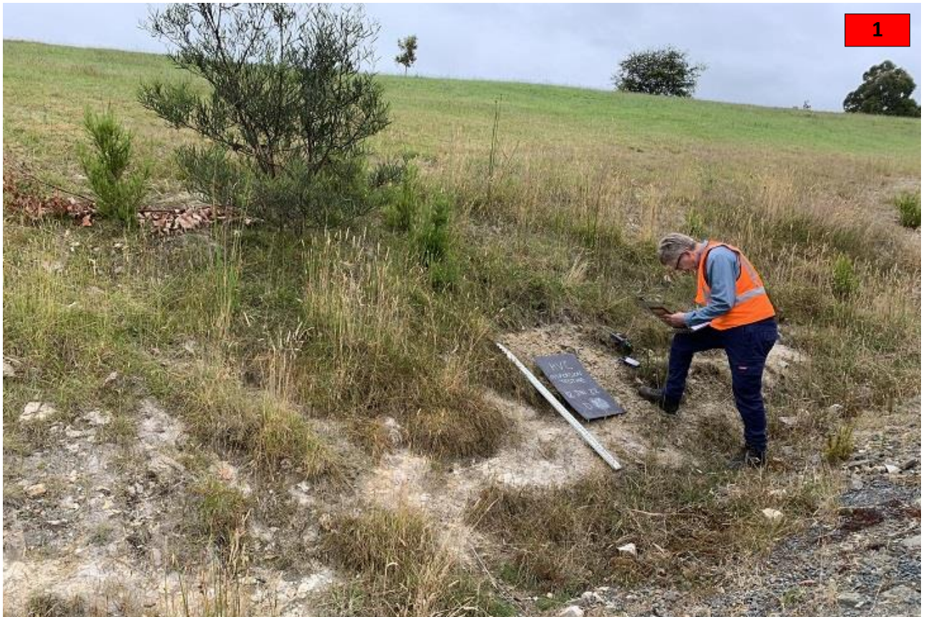
Site D20 (above). Massive rippled-marked Permian-age sandstone. Poor topsoil development, silty clay where present. Sand 10%, silt 20%, clay 70%. Tested sample: Emerson Class No. 1 (complete dispersion).
