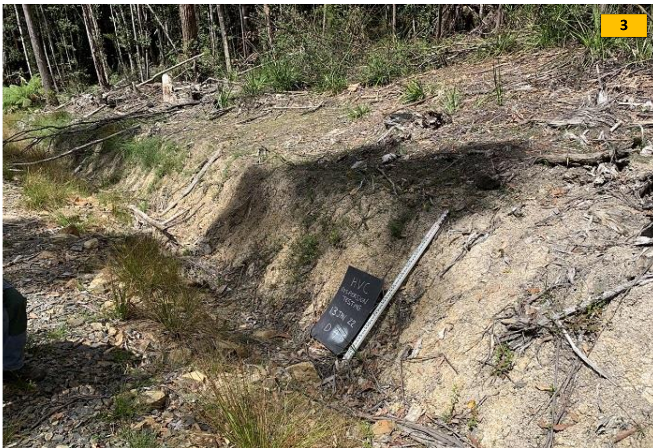
Site D48 (above). Orange-white coloured Permian?-age siltstone weathered to a sandy silt. Silt 80%, sand 10%, clay 10%. Tested sample: Emerson Class No. 3 (slight dispersion).
