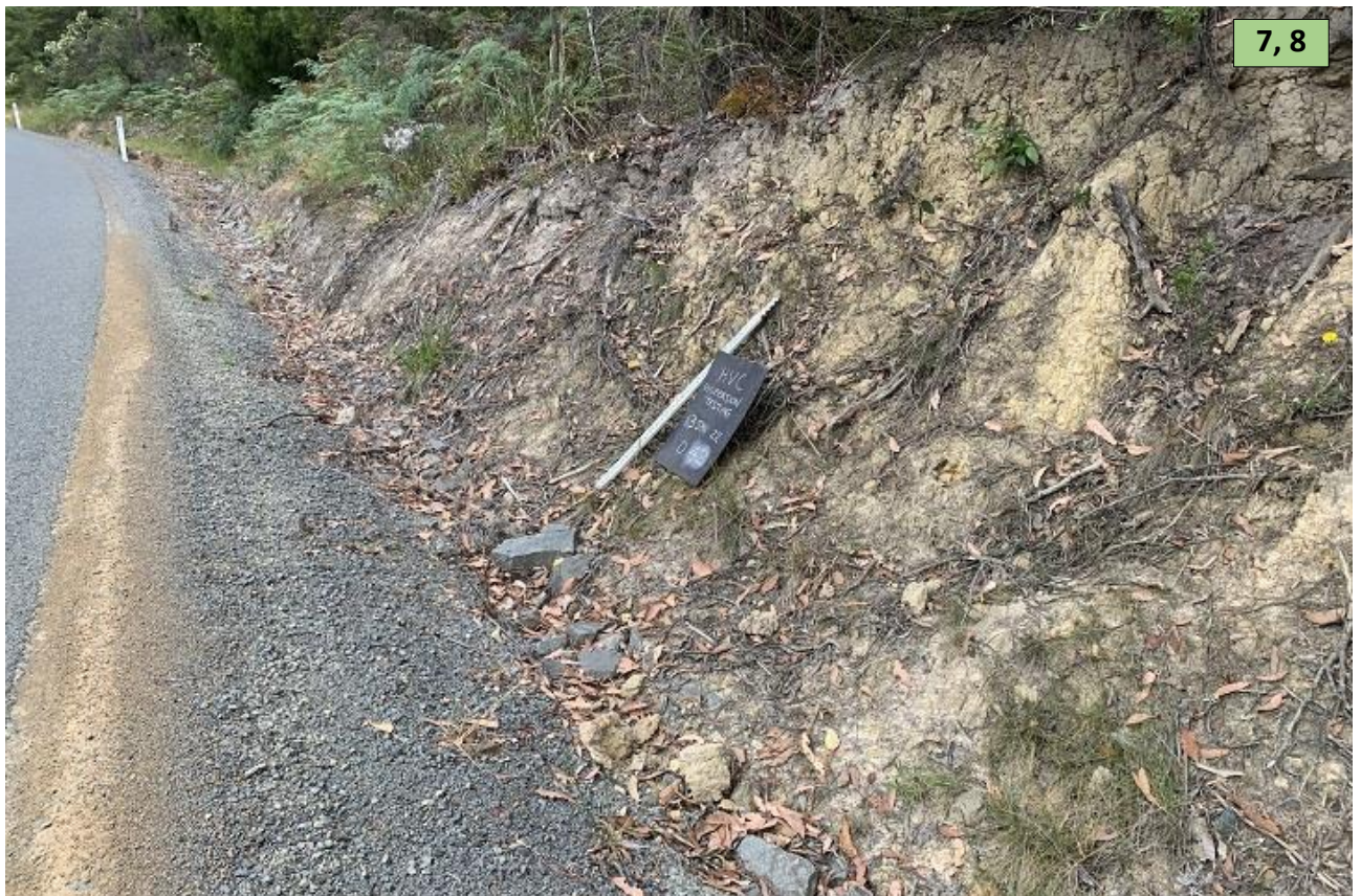
Site D42 (below). Light-brown coloured Triassic-age siltstone weathered to a sandy silt. Silt 80%, sand 20%. Tested sample: Emerson Class No. 7 or 8 (no dispersion).
