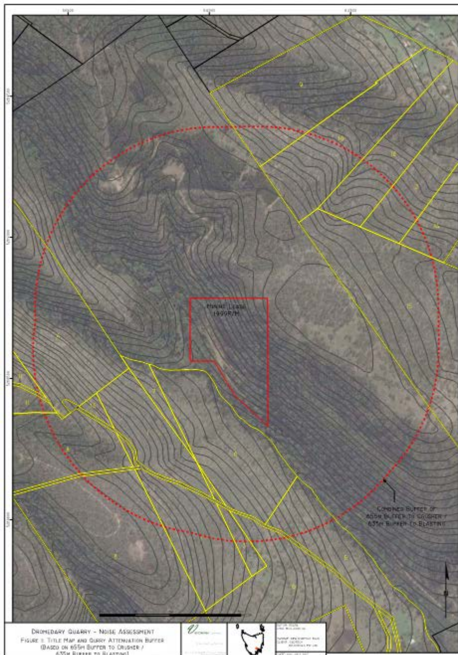
Figure 12 - Noise and vibration limits shown by the dotted line which will form the boundary of the Attenuation Area overlay over Dromedary Quarry
