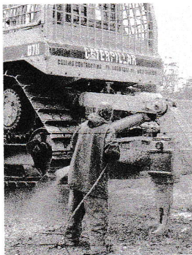
A high pressure water spray removes general accumulation of soil. Note how tracks have been lifted off the ground.
